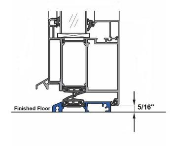
7. Remove gasket to access the mounting groove.
